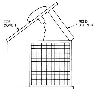
Fig. 16 — Pivot and Support Top Cover
